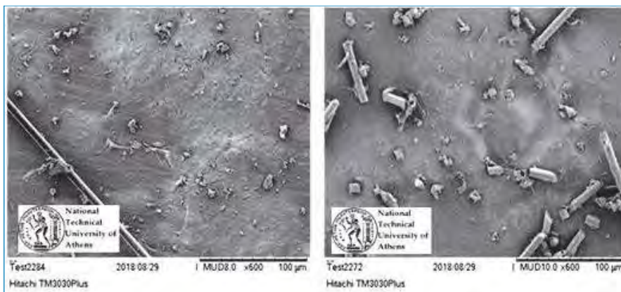
SEM micrographs : Composites surface with CNT/CNF non weathered (left) and weathered (right). Cells observation on the surface of the composites.
