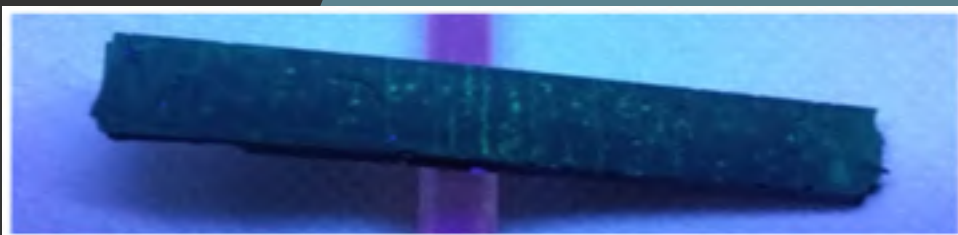
Micro-cracks revealed with UV light
