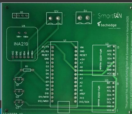
Techedge printed circuit realized in order to implement Arduino Nano together with IoT sensors to acquire signals from fan devices.
