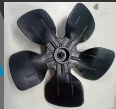
Axial Impeller moulded with PP modified with CNTs
