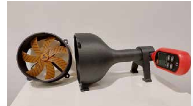
Axial cooling fan prototype with shape morphing composite blades for thermal managing applications
