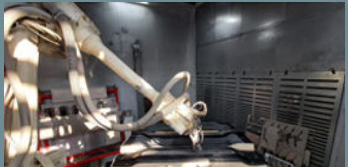
Figure 1: Smartfan front wing manufacturing with a semi-automatic preform made with a vacuum bench
