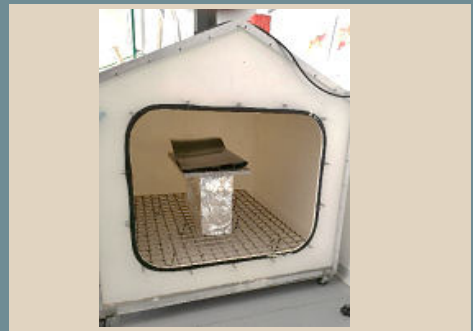
Figure 11. Modified CFRP specimens (intended for the DAL demonstrators) during the aging process.
