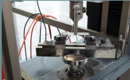
Figure 6. Mechanical - flexural - measurements setup.
