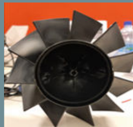
Figure 2: Injection molded fan wheel with selected Smartfan material
